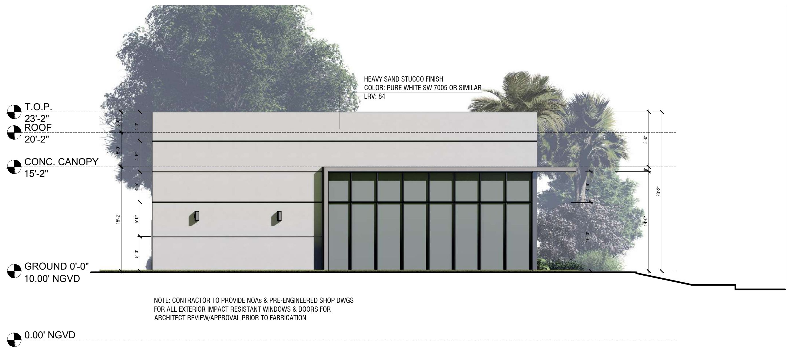
2 SOUTH ELEVATION - SOUTH BUILDING 1/8"=1'-0"
