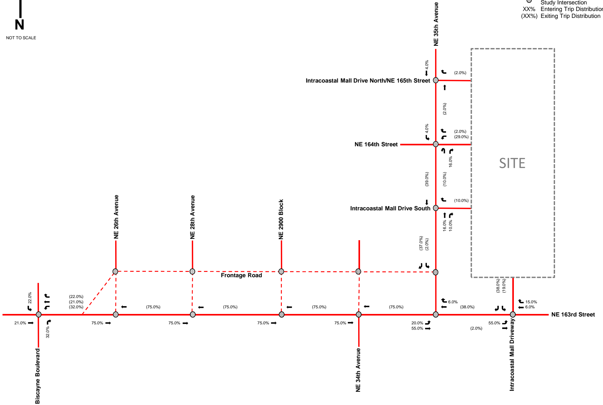
Figure 5 Peak Hour Project Trip Distribution with Improvements Intracoastal Mall Redevelopment North Miami Beach, Florida
