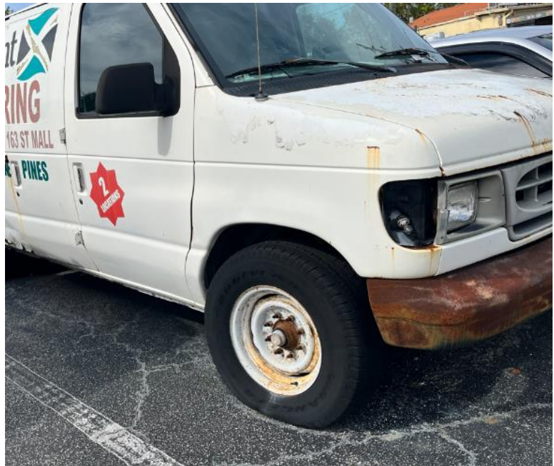
FIGURE 2: EXAMPLE OF COMMERCIAL VEHICLE IN DISREPAIR, WITH SEVERE RUST IN SEVERAL PLACES, BUSTED TURN SIGNAL, ROTTING TIRES, FADED MARKINGS, AND VEHICLE TAG EXPIRED SINCE 2019.
