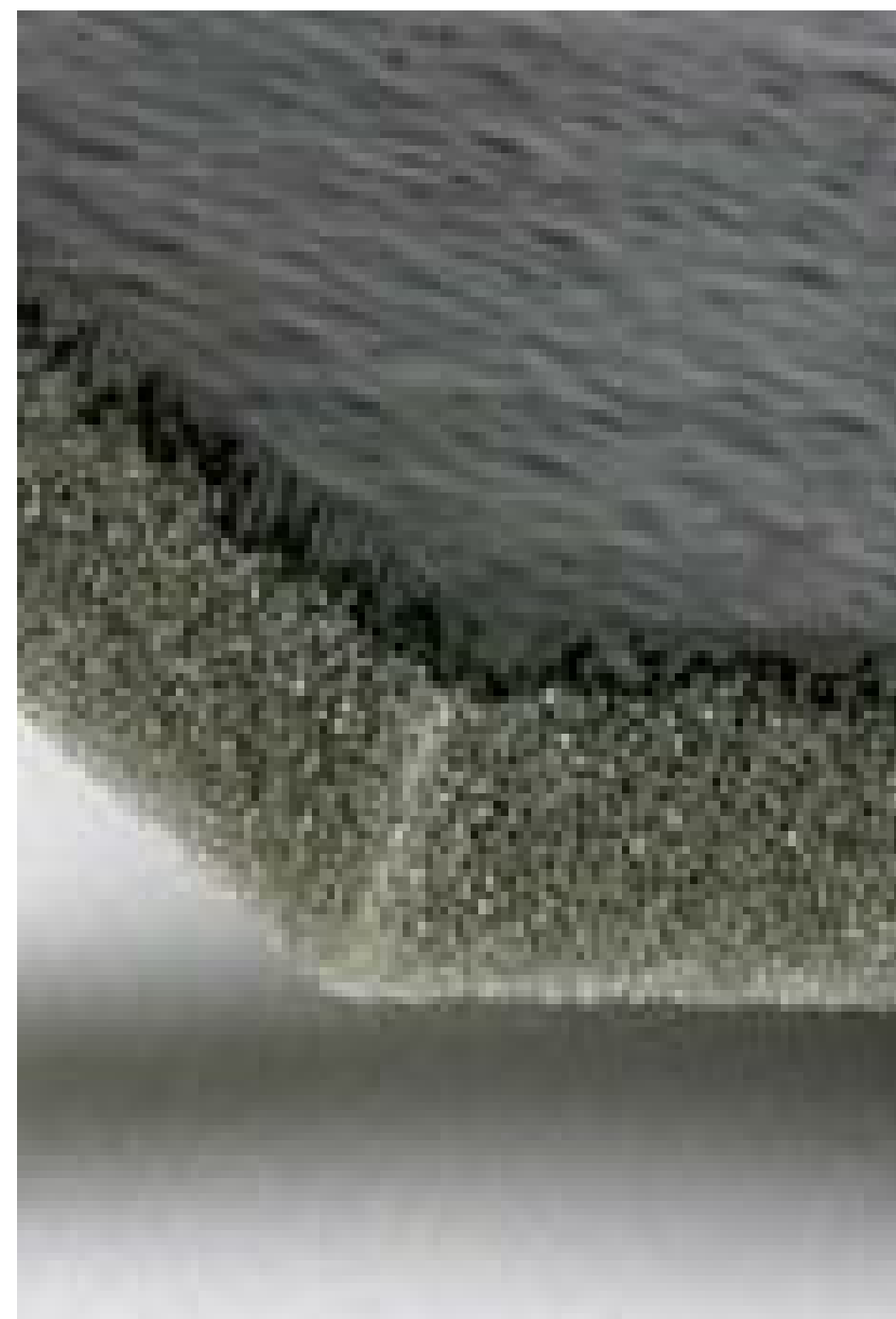
3. PARKING LIFTS GENERATOR ENCLOSURE: SOUNDPROOFING COMPOSITES / NOISE INSULATION. (SOUNDPROOFING MEMBRANE AND ACOUSTIC GRADE, POLYURETHANE FOAM.)
