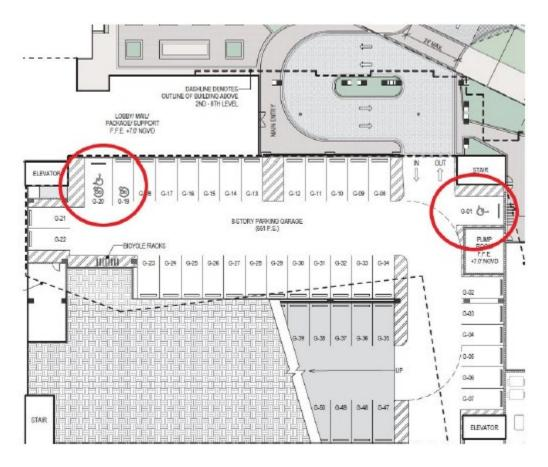
Response: Please refer to latest sheets SP-1, and A.202 to A-2.05 for revised ADA spaces markings. Typical dimensions for ADA spaces have also been added for clarification.
